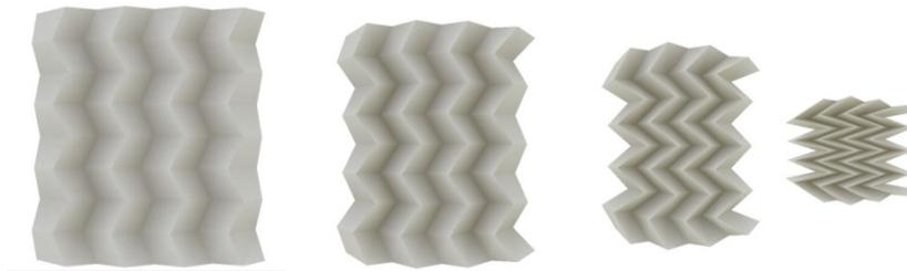
Figure 3: Various deployable states of a Miura pattern. Computer simulations created using FreeForm Origami by Tomohiro Tachi.
